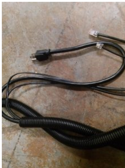
Cables With Pre- Attached Wire Loom
